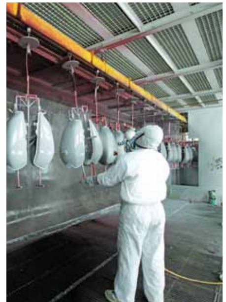
AkzoNobel coatings being applied to motorcycle fuel tanks
